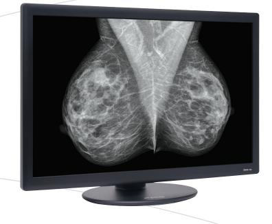
The **Dome S10** display enables the next great advancement for mammography with the brightness and speed for tomosynthesis. The S10 grayscale display is capable of showing two 5MP images for back-to-back chest wall reads.
